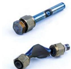
*Burst cladding after oxidation*
