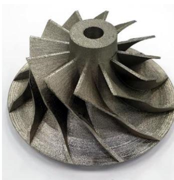
Example of a 3D model component elaborated by additive manufacturing that will be functionalized (diameter ~10 cm)
